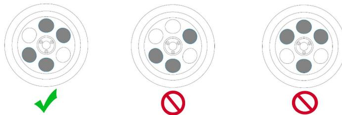
**!** Rotor imbalance may cause major damage to the rotor and centrifuge. Never attempt to introduce liquids into the tube inserts.
